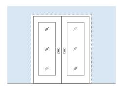
Flush pulls can be 60mm from leading edge to flush pull edge for both doubles and singles. Improving from the market norm of 100mm.
